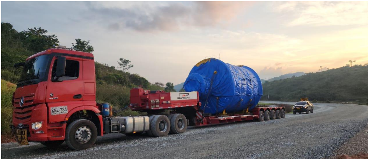
New mill transport and offload at Segovia
